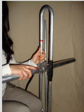
Slide elements onto boom and tighten U-bolts.
