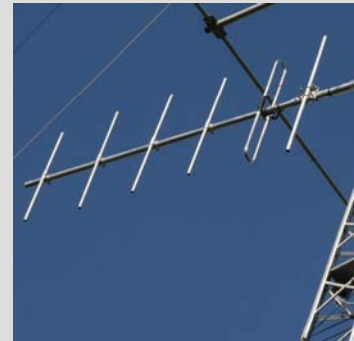
VHF YAGI fully assembled and installed
